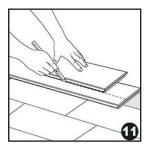
Before laying the final row, measure and saw the board accordingly. Leave 8 to 10 mm / 1/3 to 3/8" gap between the board and the wall to allow for any expansion.
