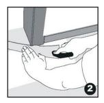
Door Frames: saw the door frame, resting the flat edge of the saw against a board so that the board can fit underneath.
