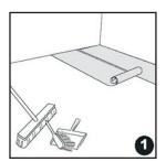
To start, ensure that no damage has been done to the flooring during transportation. After cleaning the floor surface you can roll out the plastic sheet & underlay material. The plastic should overlap by at least 20 cm/8".
