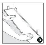
Lay the first board against the left wall, with the tongue-side towards the wall. Make sure you leave a space of 8 to 10mm/ 1/3 to 3/8", to allow for expansion. If the wall is uneven, the boards should be sawn & adapted to the contour of the wall.
