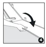
Insert the end of the second board into the end of the first, pressing them together and pushing gently down towards the floor. Complete the first row in the same manner.
