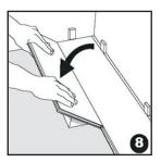
Place the sawn board by tilting it against the first row board exert pressure and, at the same time, press down towards the floor. Place a triangular wedge under the board.
