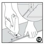
Pipes. Measure the diameter of the pipe and allow for an extra 10 mm / 3/8" leeway. After cutting the board as illustrated in the diagram below, lay the board & the part sawn off.
